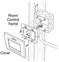
After securing the user interface frame to the junction box, snap the cover onto the frame.
